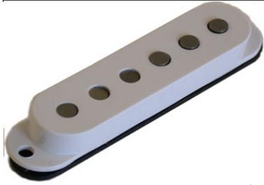
Staggered polepieces with Flat top Alnico V magnets. Middle pickup is reverse wound / reverse polarity. Bridge pickup is slightly overwound for better balance. Classic “Strat” style sparkle without sounding thin. Contemporary stagger better suited to today’s string gauges to give superior string to string balance.
